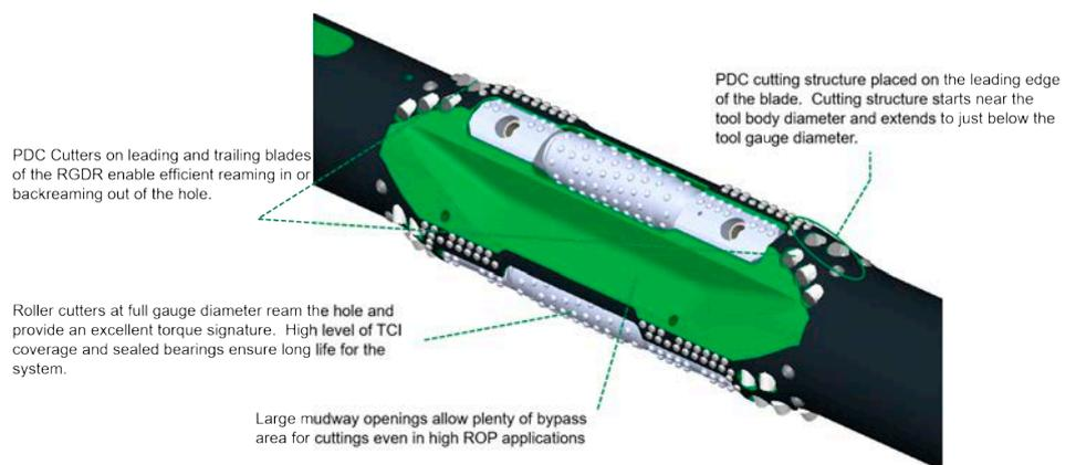
Figure 4. Roller GunDRILL Reamer.
