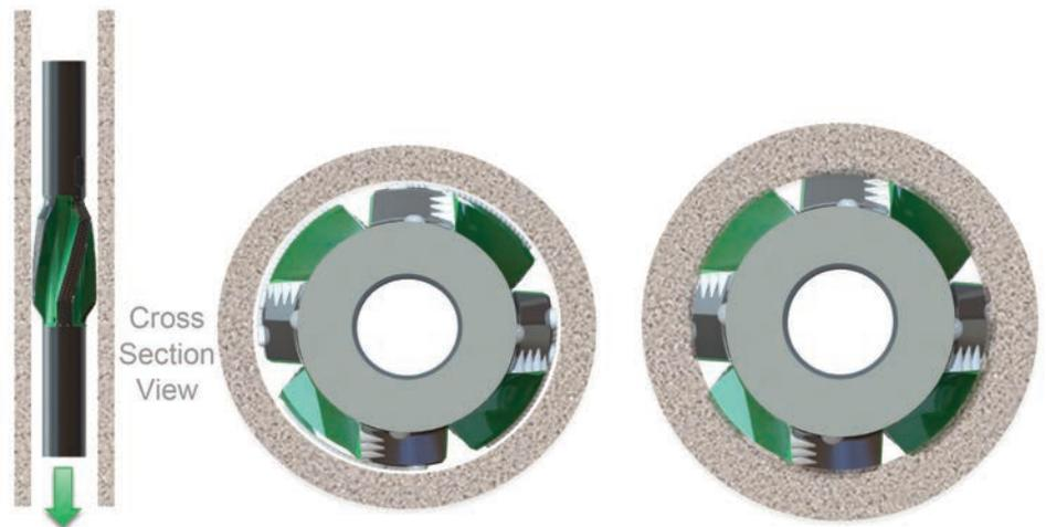
Figure 3. Cutting structure engagement.
