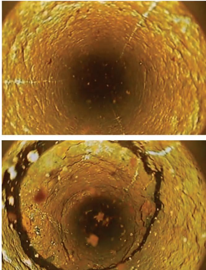
Figure 1. Conditioned wellbore (top), common wellbore (bottom).
