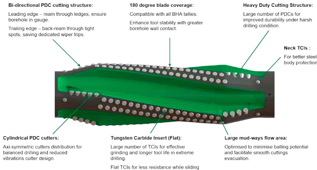
Figure 2. GunDRILL Reamer.
