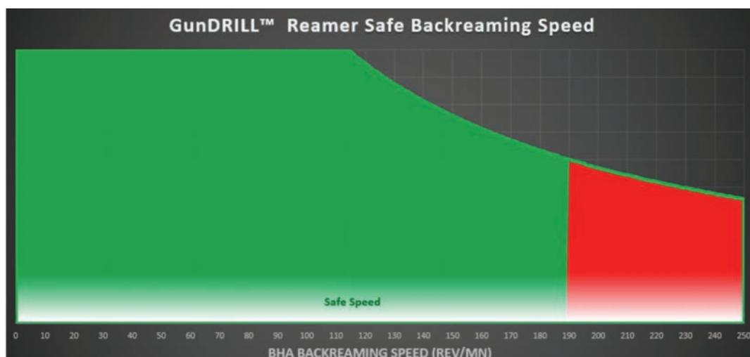
Figure 5. Backreaming RPM guidelines.
